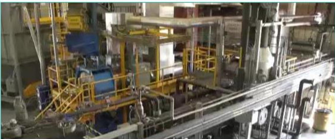
2014 – Gen 6: Continuous processing: Plastic-to-oil
